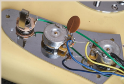
The lead circuit's 1meg-ohm pots are full size – plus, note that added resistor on the tone control
